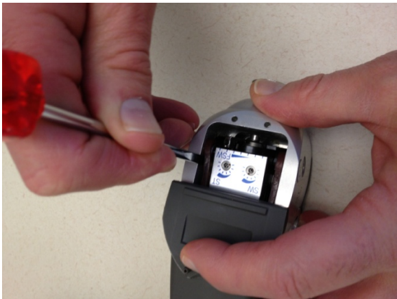
Fig. 2 Removing the springs from the distal attachments.
