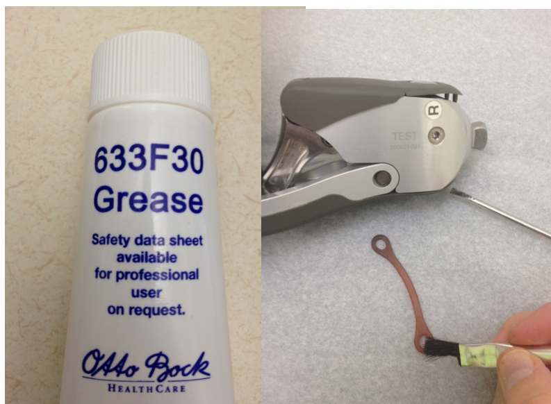
Fig. 4, Applying grease with a brush
