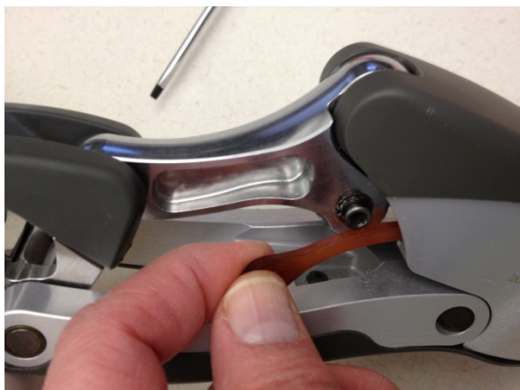
Fig. 5, Slipping the band into place
