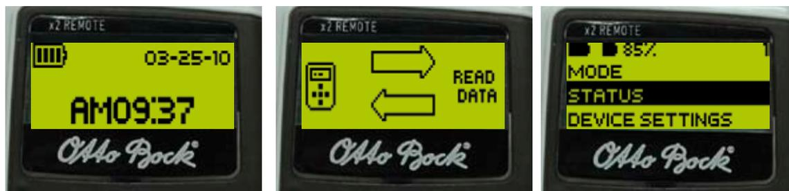
1. Press the enter button to activate the remote control. The start-up screen with the date, time and charge status of the remote control is displayed. Without additional input, the remote control turns off automatically after 5 seconds.
