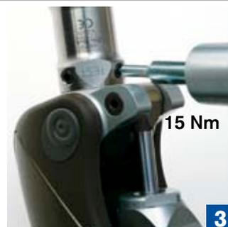
Use a 710D4 torque wrench with a 710Y2=4 hex bit to tighten the screws alternately, in several steps increasing the torque slowly, until the prescribed torque is reached:
