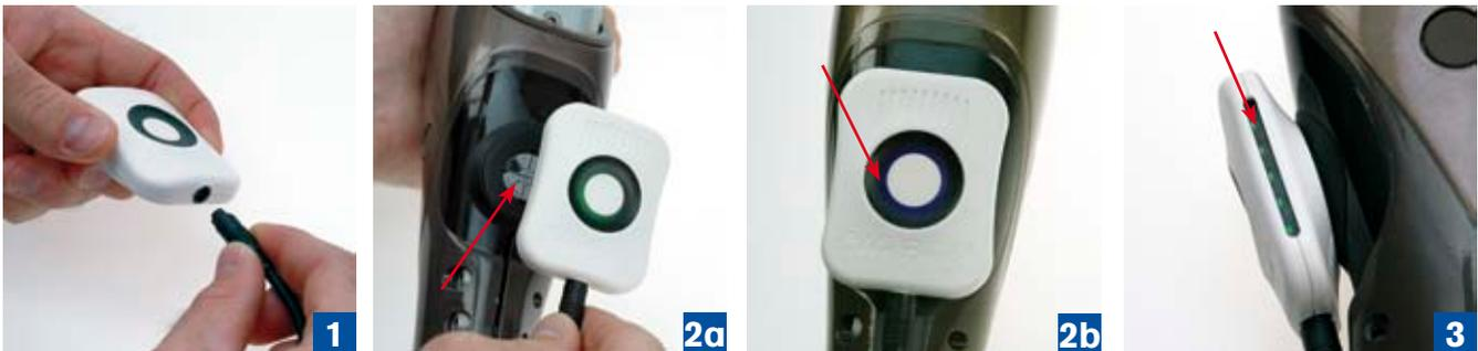
1. Connect the power cord to the charger with correct polarity (Figure 1).
