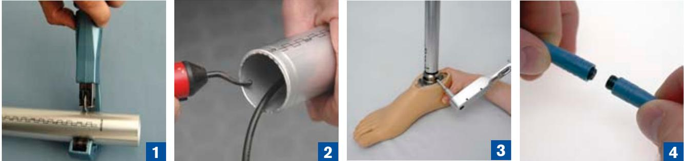
1. Determine the length of 2R20/2R21 AXON Tube Adapter required with the configuration software X-Soft.
